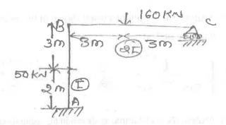
(c) Analysis pin jointed structure as shown in fig. hence find the member forces using stiffness method. The area of cross sec of each member is 2000 mm<sup>2</sup> take  $E = 200 \text{ kN/mm}^2$ .
